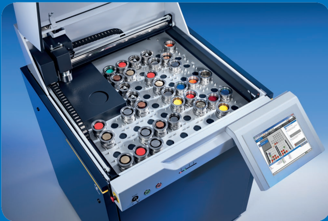
60 Pos Sample Cup Loader for heavy samples and XRF 2 mapping with HD camera
